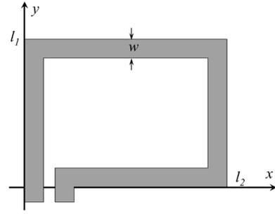
Fig. 6. One-turn rectangular PCB winding.
