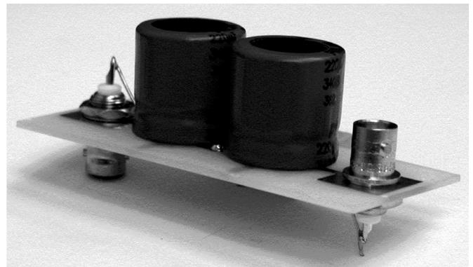
Fig. 9. Implementation for two  $220 \mu\text{F}/250\text{-V}$  electrolytic capacitors.
