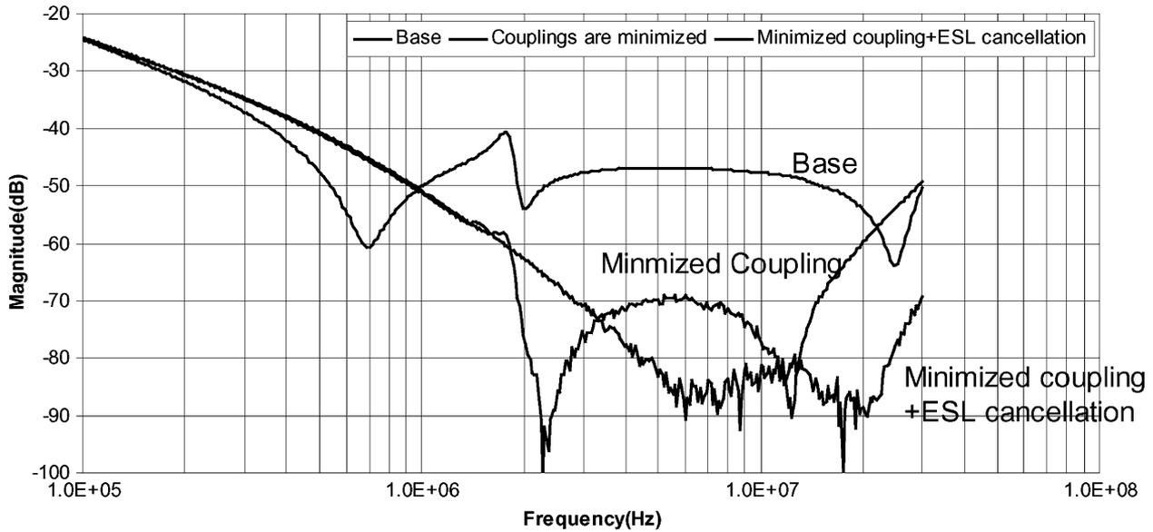
Fig. 16. Comparison of insertion voltage gains for a  $\Gamma$ -type filter.
