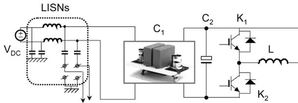
Fig. 19. DM noise measurement setup for a prototype with film capacitors.
