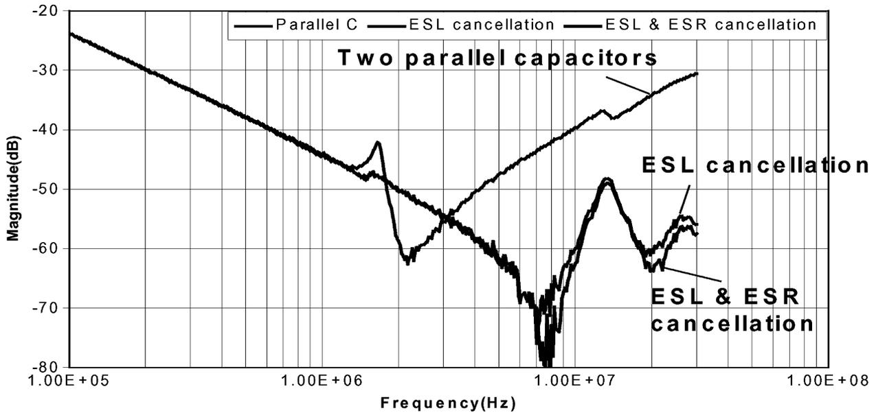
Fig. 13. Comparison of insertion voltage gains for the prototype with film capacitors.
