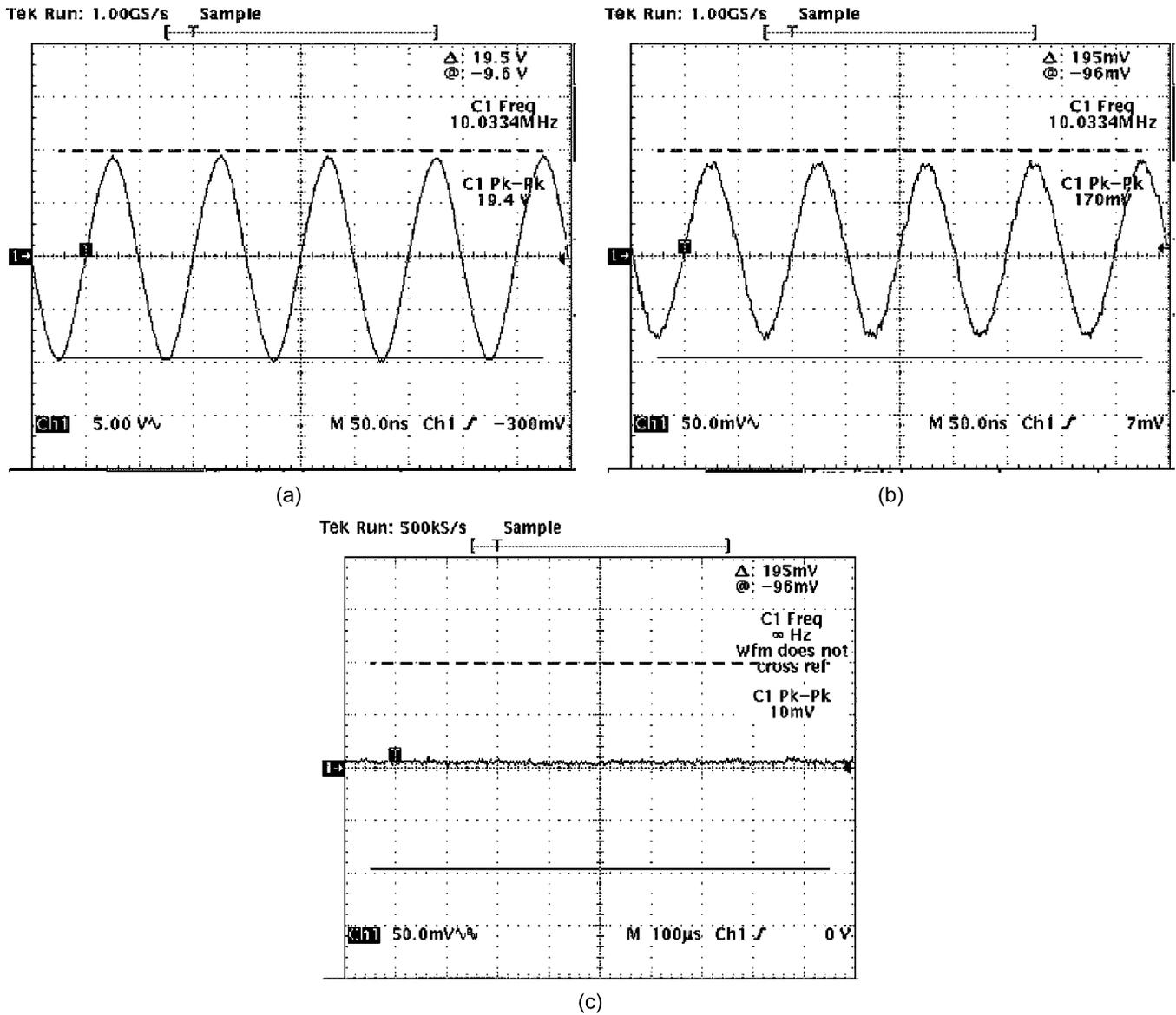
Fig. 11. Comparison of measured results for the prototype with film capacitors. (a) Input voltage ripple. (b) Voltage ripple of two parallel capacitors. (c) Voltage ripple of ESL cancelled capacitors.
