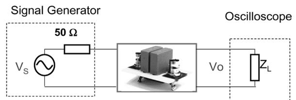
Fig. 10. Equivalent measurement setup for the prototype with film capacitors in time domain.
