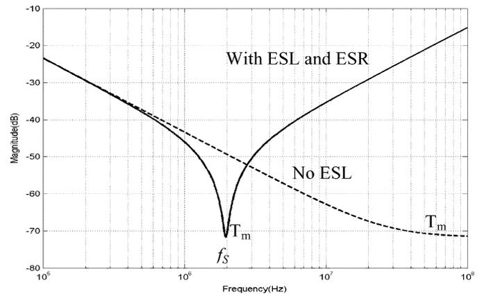
Fig. 2. Insertion voltage gain curves of capacitors.
