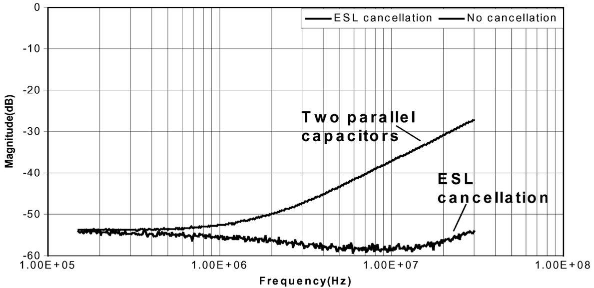
Fig. 14. Comparison of insertion voltage gains for the prototype with 220- $\mu$ F/250-V electrolytic capacitors.
