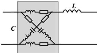
Fig. 15. Application for a  $\Gamma$  type EMI filter.
