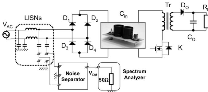
Fig. 17. DM noise measurement setup for the prototype with electrolytic capacitors.
