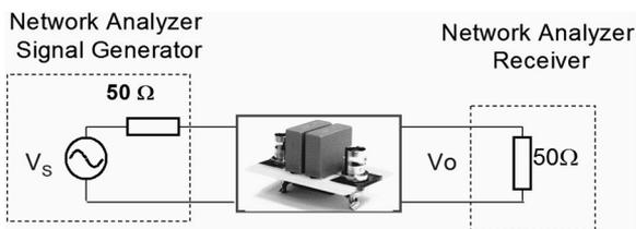
Fig. 12. Equivalent measurement setup for the prototype with film capacitors in frequency domain.
