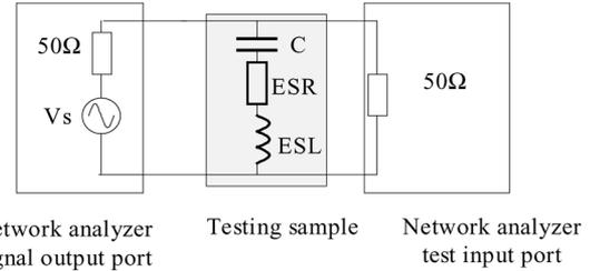
Fig. 1. Setup for evaluating the insertion voltage gain of a capacitor.
